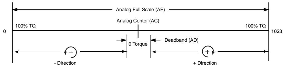
Figure 8.8: Analog settings for torque mode
