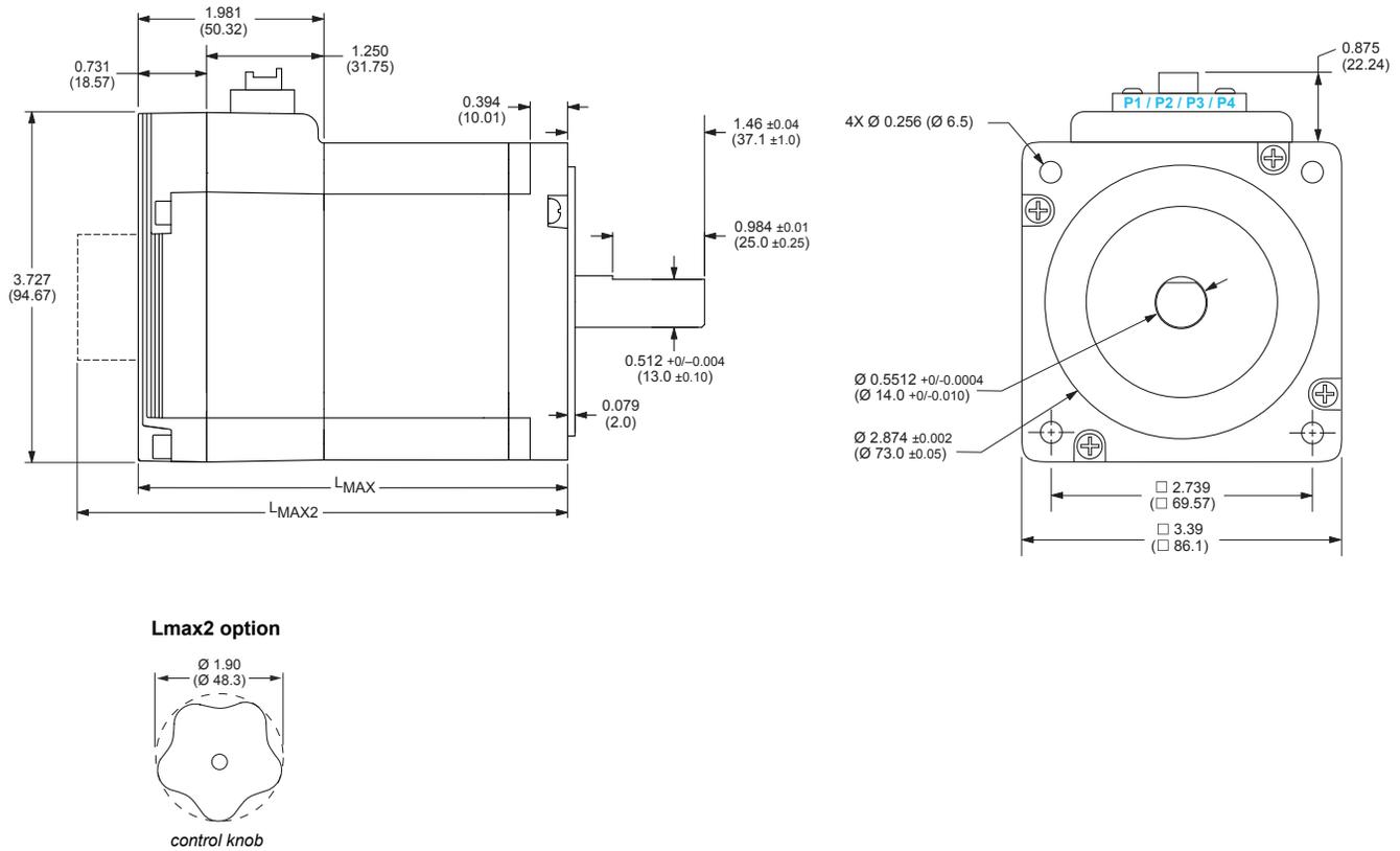
Figure 3.2: MDrive 34 Hybrid dimensions [inches (mm)]
