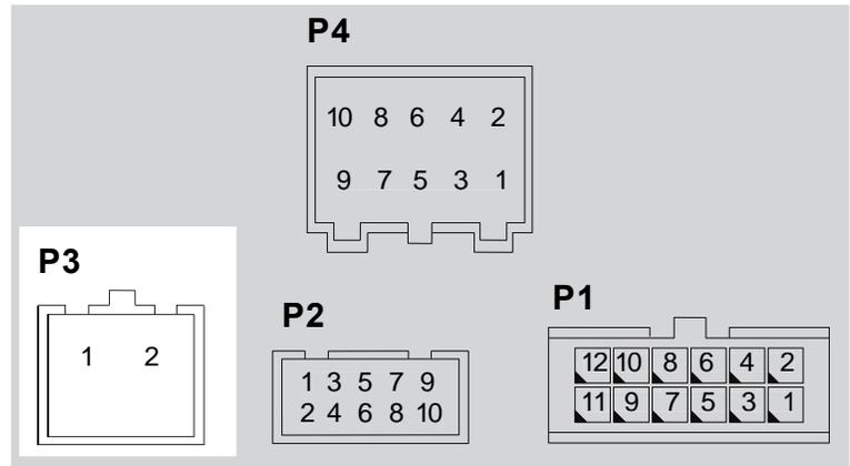
Figure 6.2: Pin Assignment supply voltage
