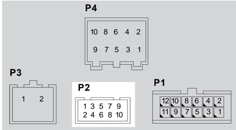
Figure 6.11: Communications interface pin assignments
