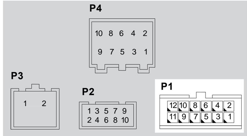
Figure 6.4: Multifunction interface pin assignments
