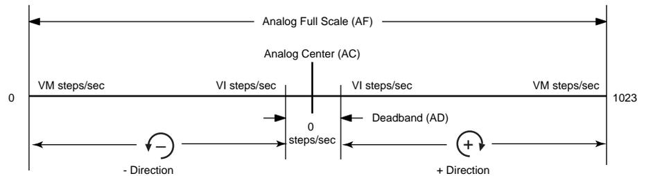
Figure 8.10: Analog settings for speed control mode
