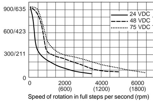
Figure 3.6: Speed torque curves
