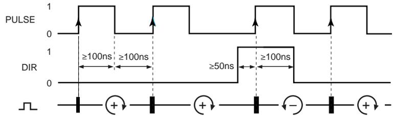
Figure 8.4: Step/direction signals and timing
