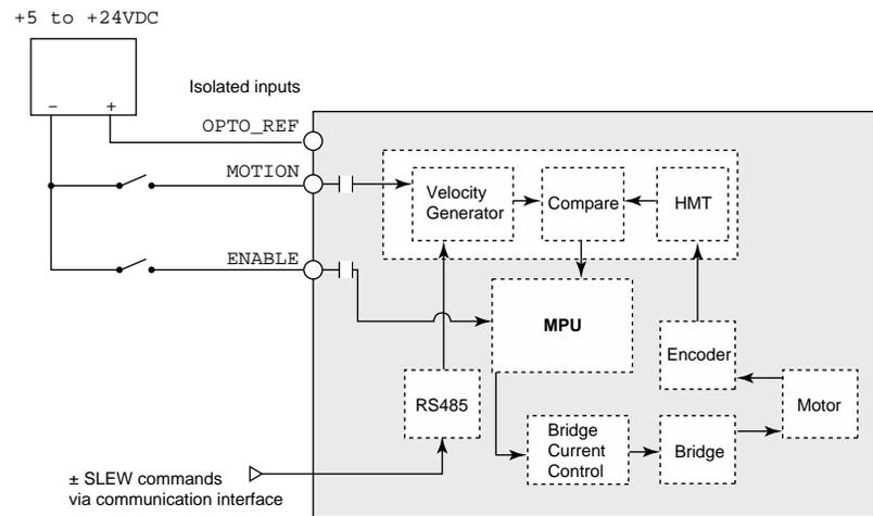
Figure 8.11: Speed control mode block diagram showing sinking input interface
