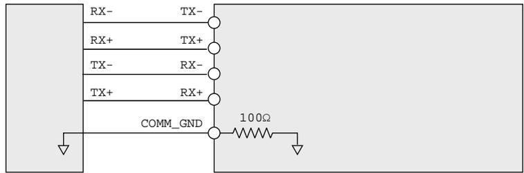
Figure 6.13: Full duplex interface, single mode (RS422).
