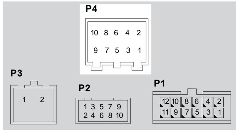
Figure 6.16: Encoder interface pin assignments
