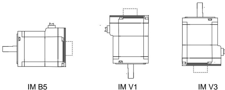
Figure 3.1: Mounting positions
