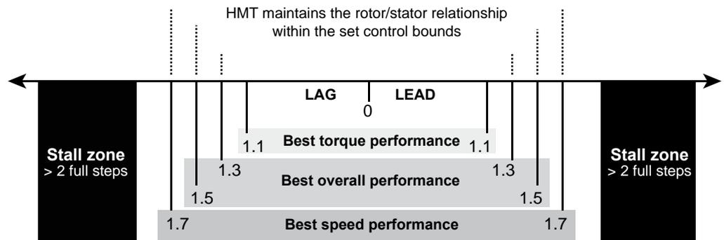
Figure 8.1: Control bounds for hybrid motion technology
