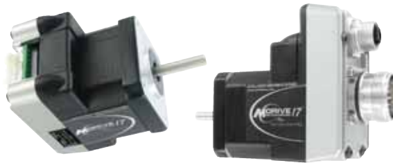
MDrivePlus MDI•17 CANopen products: integrated NEMA17 motor and controls, IP65 & IP20-rated
