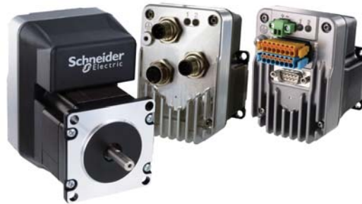
LMD•P57 Lexium MDrive Pulse/direction input products: integrated NEMA23 motor and controls, IP65 & IP20-rated
